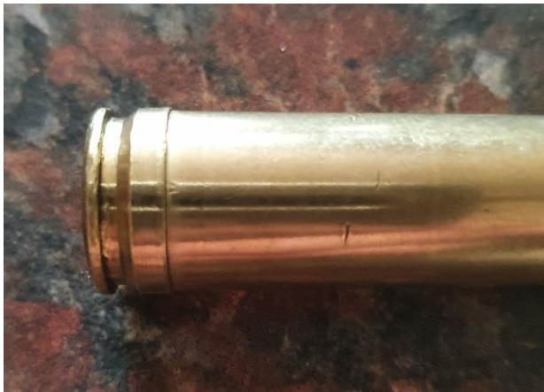
Figure 7 No groove in front of belt
