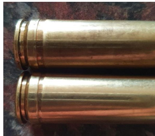
Figure 8 Groove in front of belt
